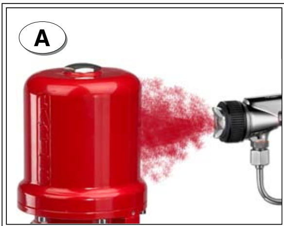
Trace of spraying a fluid at low-pressure without using air.
