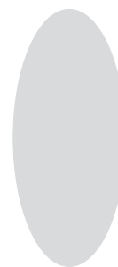
Symmetrical trace of spraying a fluid using air. No tail-end is formed.
